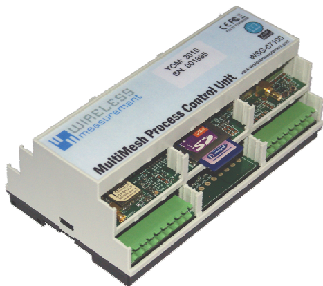
9 unit DIN (TS35) Enclosure 160mm(L) x 90mm(W) x 58mm(H)
